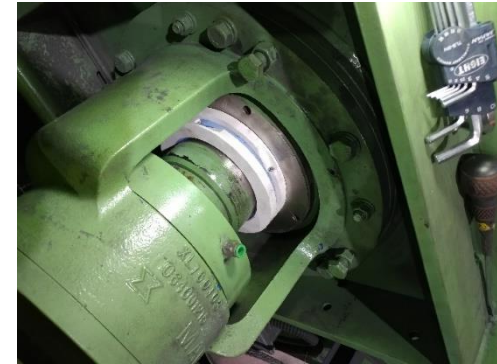
Mixing Process Mixer are used where Conductive material and Binder is added.
